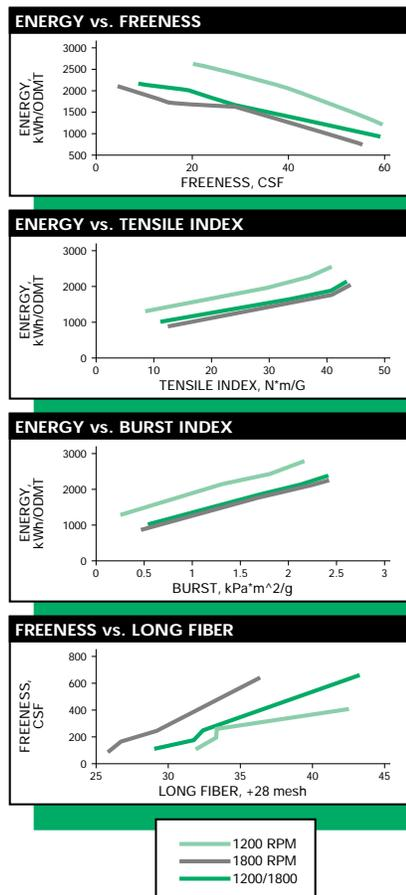
feed end only at 1800 rpm provided the same energy savings over 1200 rpm, with pulp quality relatively unaffected. In-mill operating experience has shown there are
