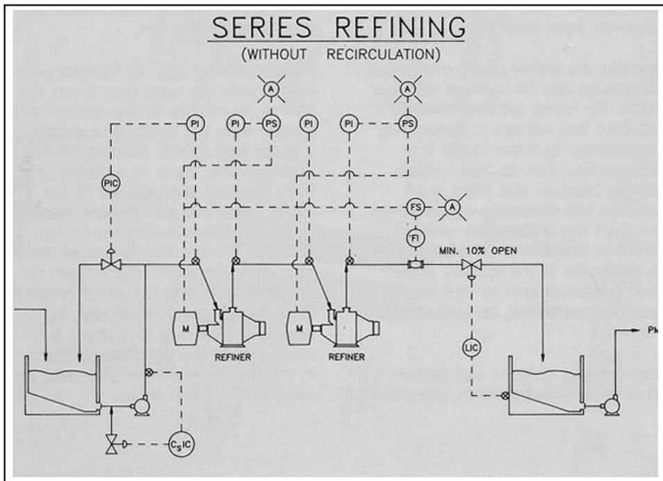
Generally, the power requirements for most grades can be attained with two refiners. For some grades, however, more than two refiners in series may be necessary. In these cases it is recommended that an intermediate chest be used so that there is no more than two refiners in series. When more than two refiners are used in series it is possible to develop excessive pressures in the system. High refiner system pressures can cause operational problems, as discussed earlier.
