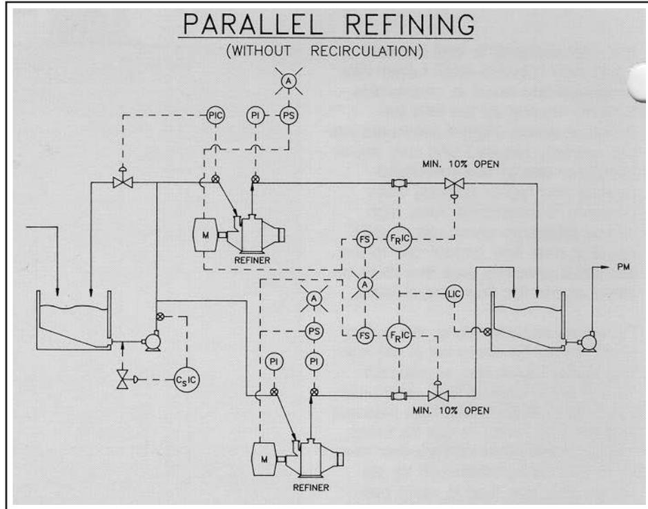
*Parallel refining (Fig. 4).* Parallel refining is generally used only when the flow requirements for the system are greater than the hydraulic capacity of a given size refiner. Parallel refining is usually the result of a desire to have identical size refiners in the same paper mill for different machine productions/grades structures. An example is linerboard machines, which may have the same size refiners on both the base and top sheet systems even though
