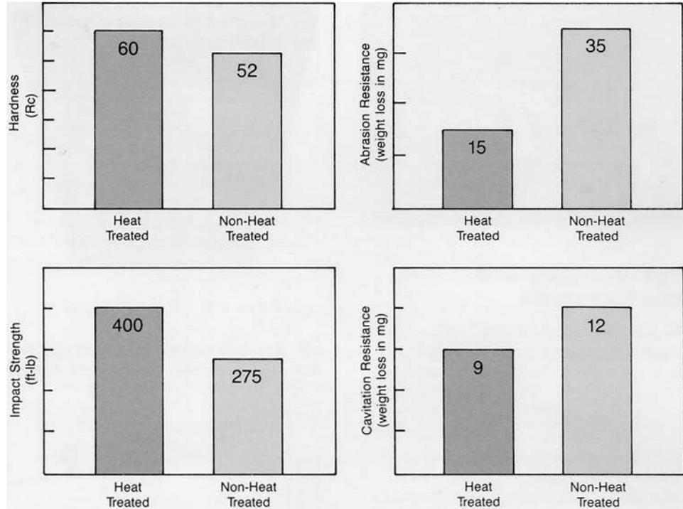
*Fig. 3: Heat treated white iron (left) versus non-heat treated white iron (right).*
