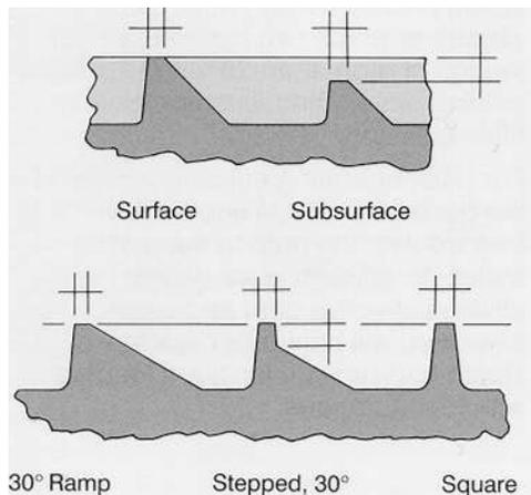
Fig. 3: The Effect of Taper
