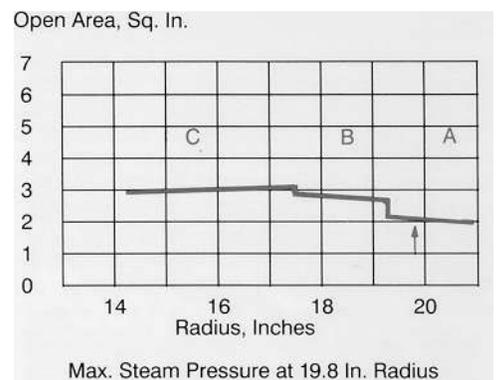
Fig. 9: Effective Open Area Curve for 42SW121 with a Compound Taper of 2" FLAT/BALANCE @ 0.010"/"
