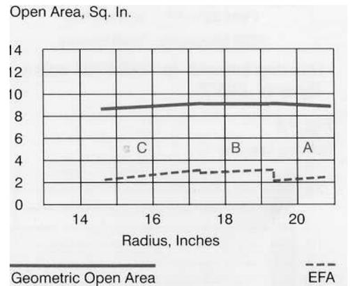
Fig. 8: Effective Open Area Curve for 42SW121 with a Constant Taper of 0.005"/"
