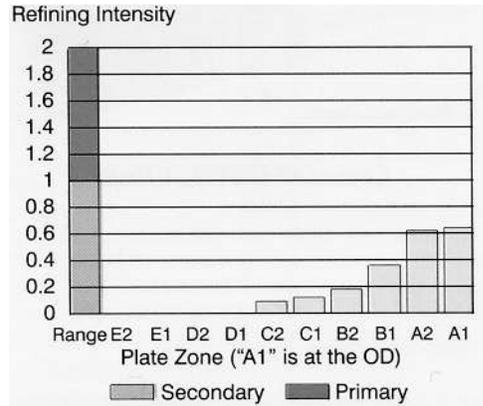
*Fig. 13: Refining Intensity for 42SW121 with a Taper of 2\"/>*
