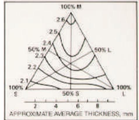
Iso-Burst lines at various chip size compositions, in  $kN/g$  at 100 ml CSF.
