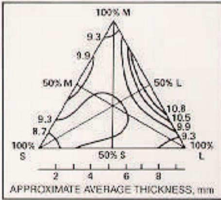
Iso-Tear lines at various chip size compositions, in  $nNm^2/g$  at 100 ml CSF.
