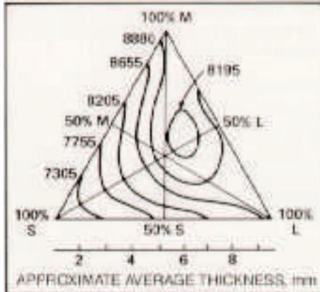
Iso-Energy lines at various chip size compositions, in MJ/ton to reach 100ml CSF.
