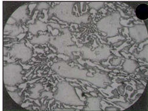
Figure 1. Typical microstructure of a high chromium white iron refiner plate. (400x magnification.)
